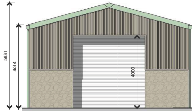
Proposed Equipment Shed, South Elevation
