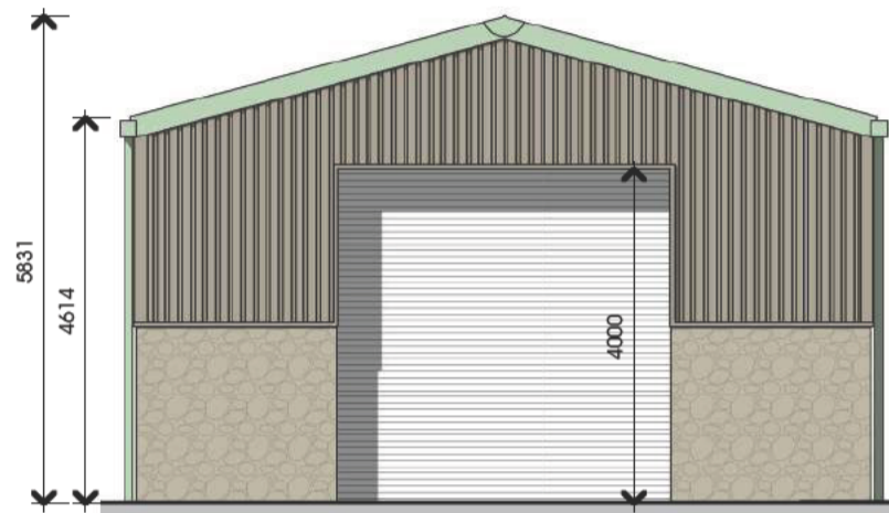
Proposed Equipment Shed, South Elevation
