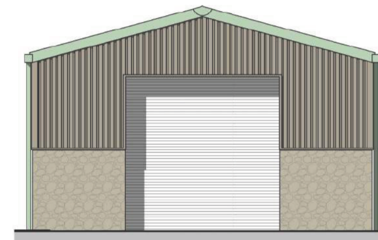
Proposed Equipment Shed, North Elevation
