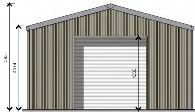
Proposed Equipment Shed, South Elevation
