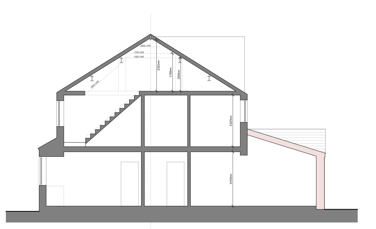
PROPOSED SECTION A:A - Scale 1:50
