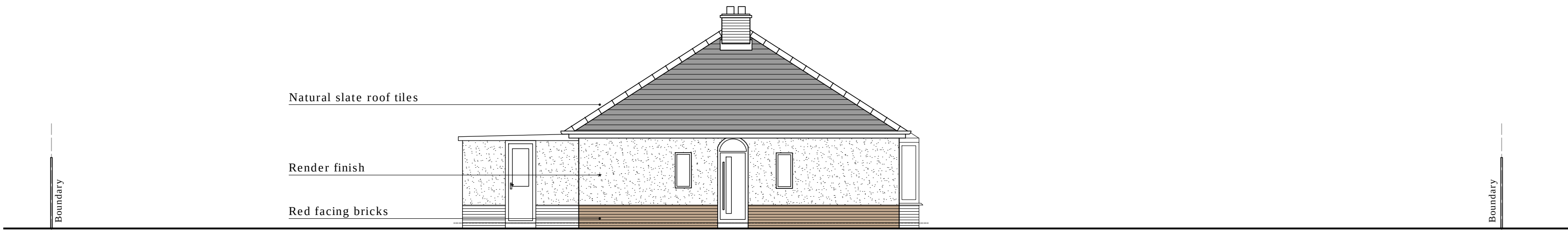
WEST ELEVATION (FRONT) 1:100
