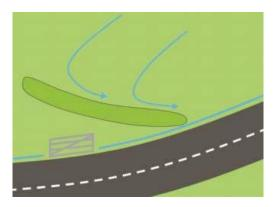
A bund is a bank created from earth, generally used as Run-off interception and storage: constructed along the contour to slow and hold back field run-off and sediment.
