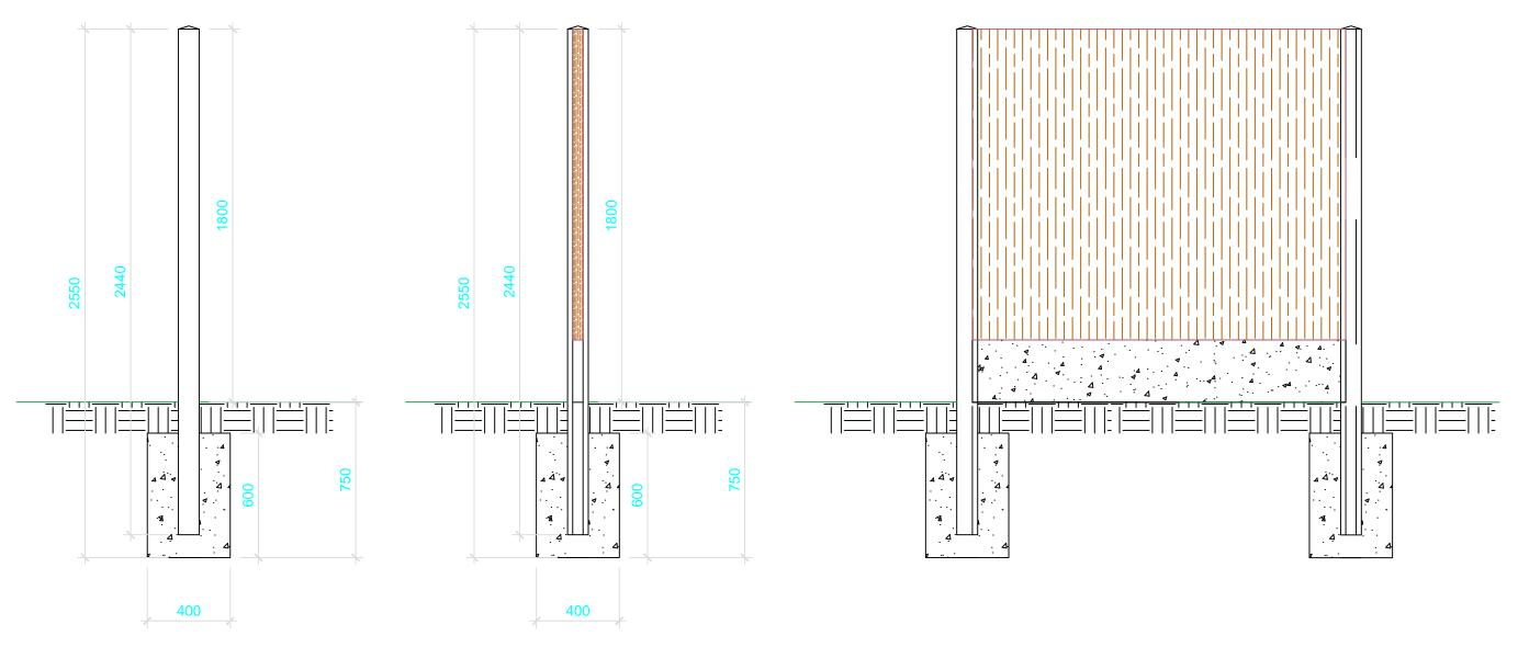
Concrete Pyramid Post 2440 x 100 x 100mm with Concrete Base Panel 1800 x 300 x 50mm and Timber Close Boarded Panel 1800 x x 50mm, set in concrete as shown. End posts to be used at the start and end of run of fencing, intermediate posts along the length ar corner posts at change of direction.
