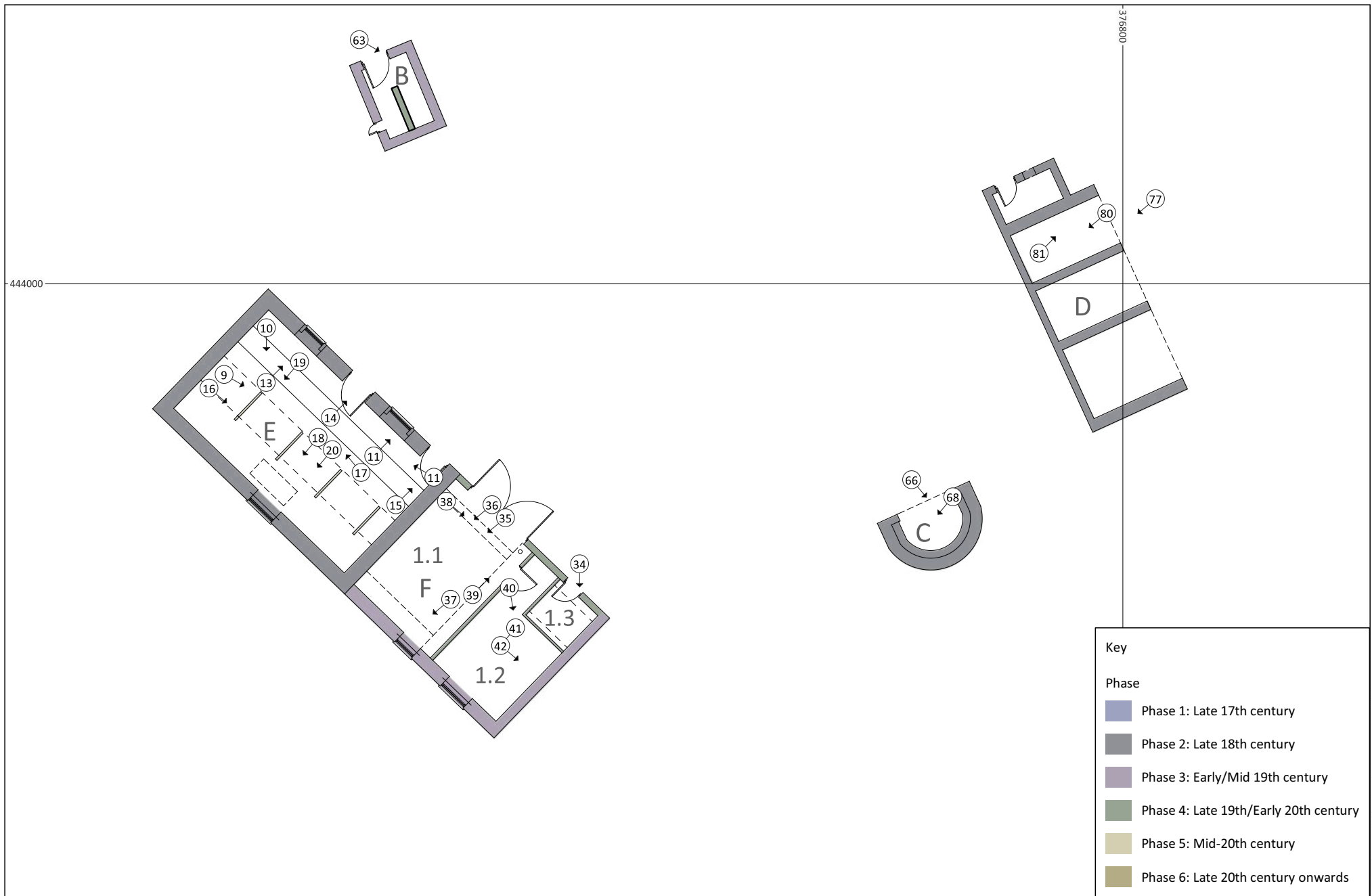
Figure 6: Phased ground floor plan of Structures B, C, D, E and F, showing location and direction of photographs (base plan provided by the client, amended where required)
