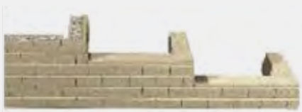
Figure 4: For a step-down that doubles as a planter, turn the wall in 2 or 3 blocks after the AB Corner Block.
