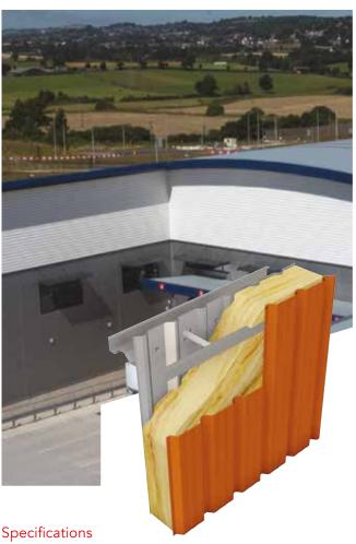
External profile EC 32-200-1000 Wall MW5 Reverse profile 0.7mm steel Colorcoat Prisma® / Colorcoat HPS200 Ultra®
