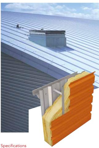
EC 32-200-1000 Wall MW5 Reverse profile 0.7mm steel External profile Colorcoat HPS200 Ultra® / Colorcoat Prisma® Spacer system Quattro Bracket and Quattro Bar Insulation 0.040W/mK Lambda insulation as standard Internal profile Euroclad EC 19-167-1000 Liner 2 0.4mm steel Fasteners, flashings, membranes, tapes, mastic and System components sealants, fabrications
