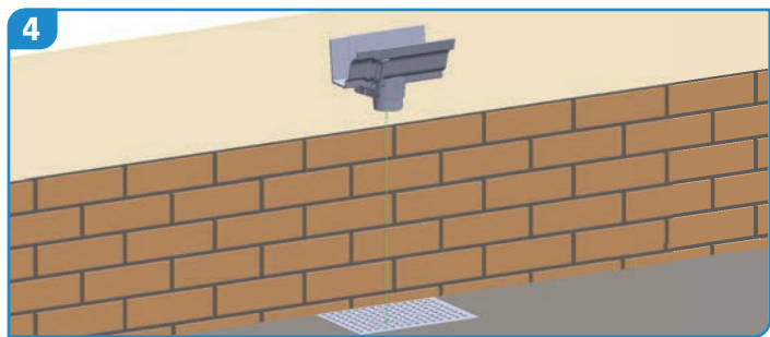
4 With the use of a plumb or laser line, position outlets over gullies and support with at least one bracket. Also include a bracket per angle (internal or external).
