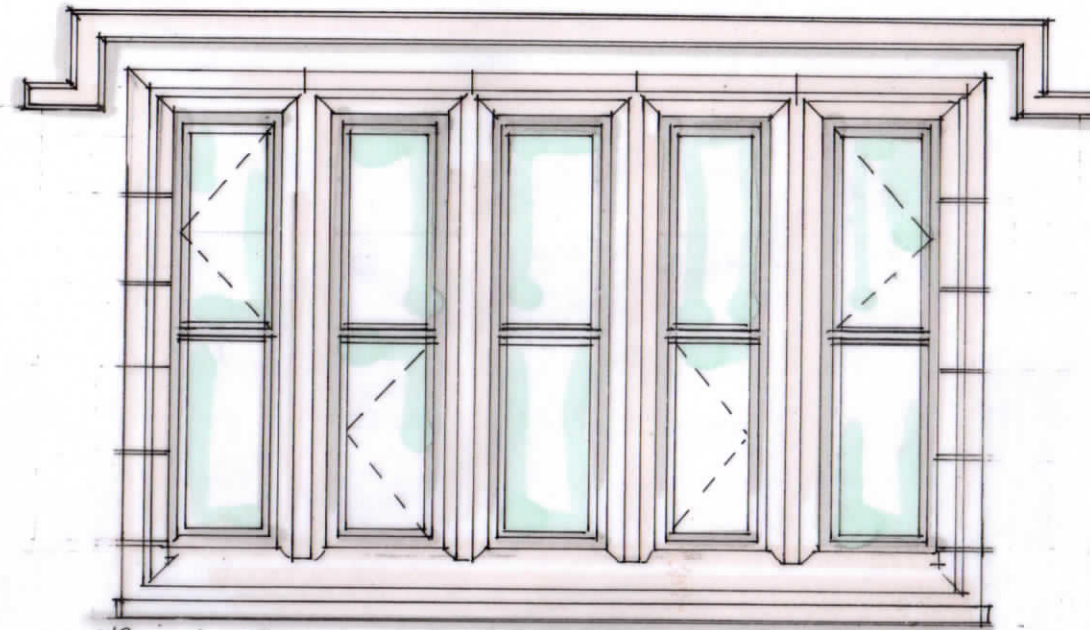
W2 - REPAIR STONE SURROUND: TIMBER CASSEMENT FITTED WITH SLIMLINE ACOYA FRAME. 14MM DOUBLE GLAZING UNIT.
