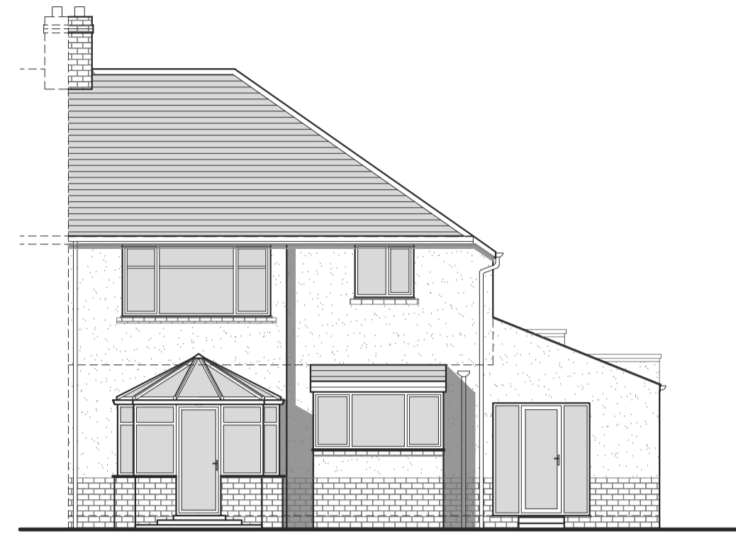
EXISTING NORTH WEST ELEVATION Scale 1:100
