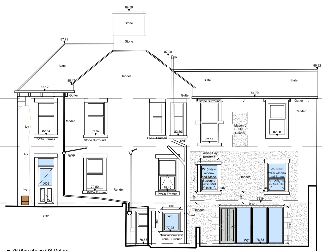
South West Elevation
