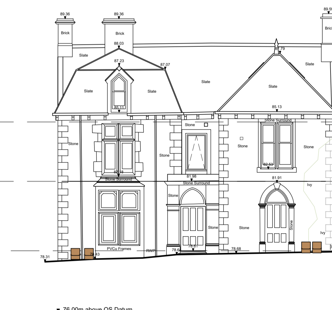
North West Elevation
