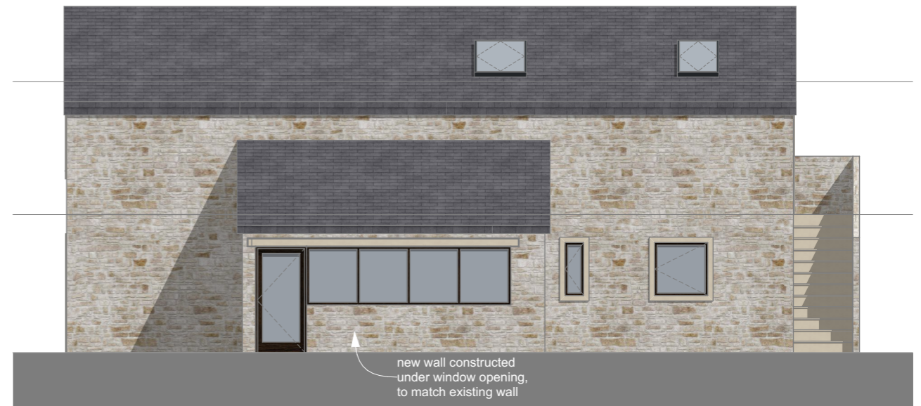
South East Elevation 1:100
