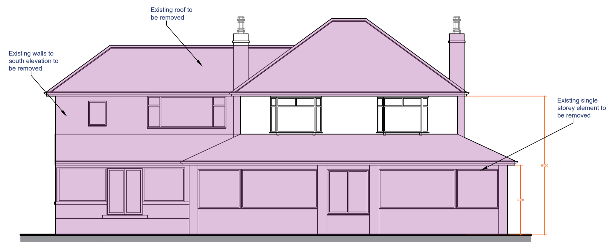
Proposed Demolition to South Elevation Scale ( 1 : 100 )
