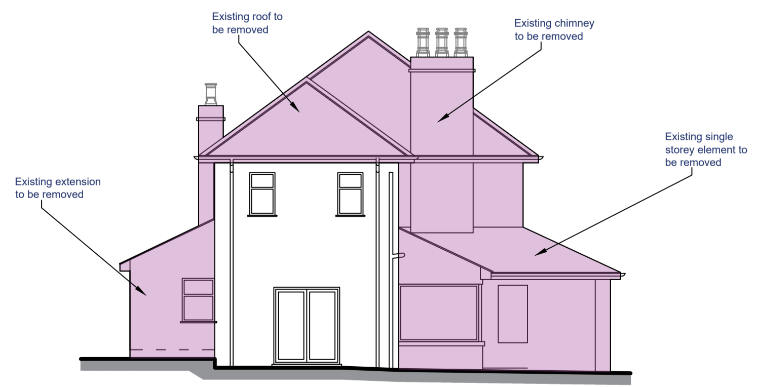
Proposed Demolition to East Elevation Scale ( 1 : 100 )
