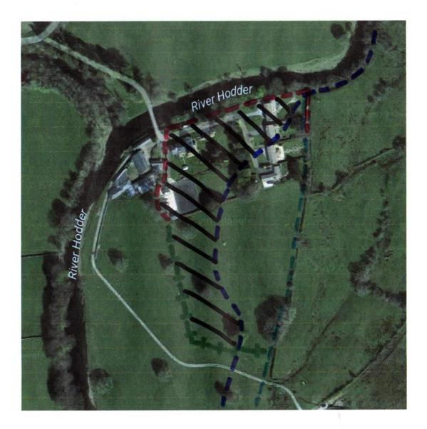
EA FLOOD ZONE 3 LINE EA FLOOD ZONE 2 LINE LINE OF RAISED EMBANKMENT WALL
