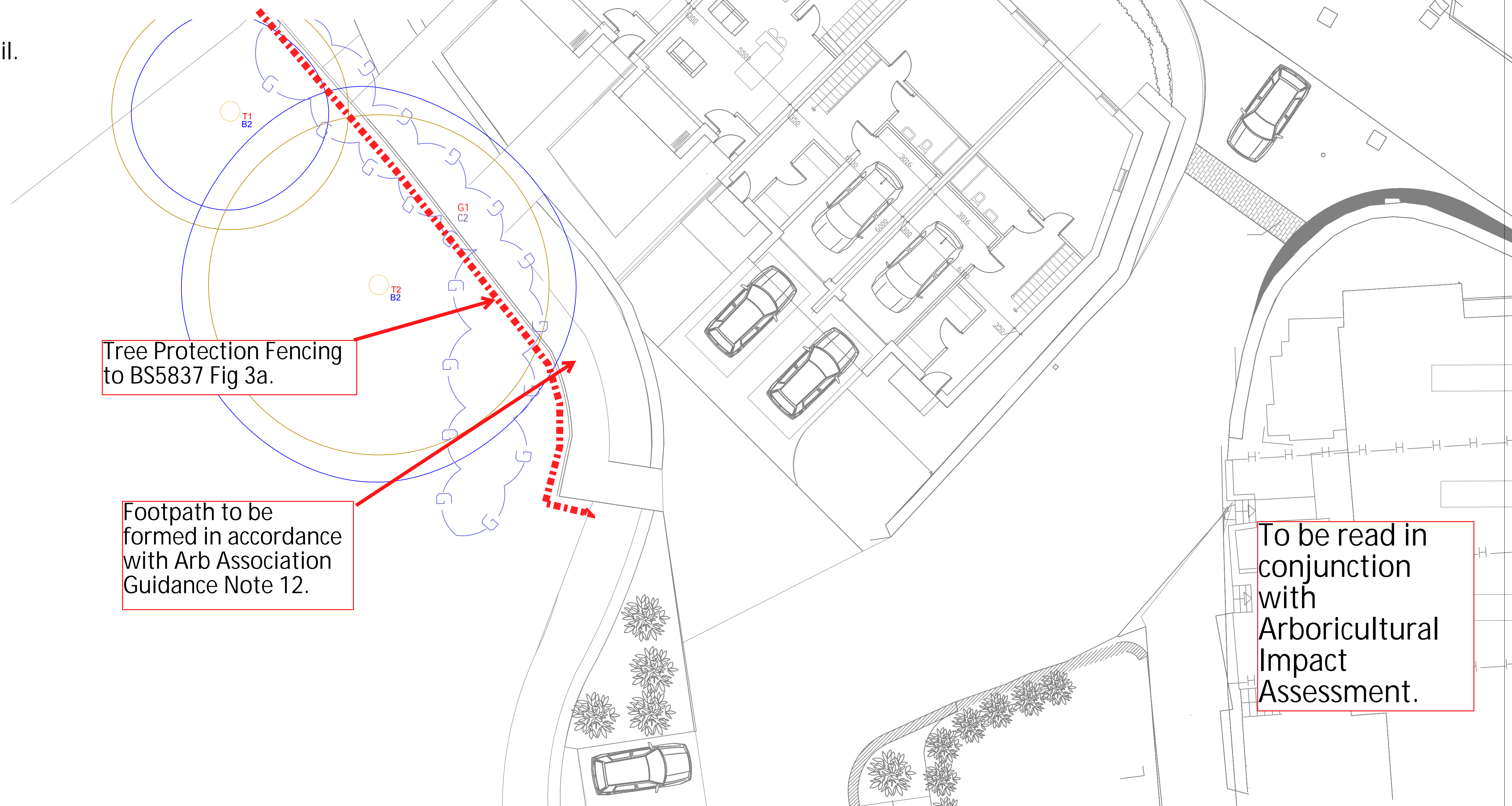
Figure 1: The basic approach to using cellular confinement systems for ground protection near trees [image courtesy of Core LP]
