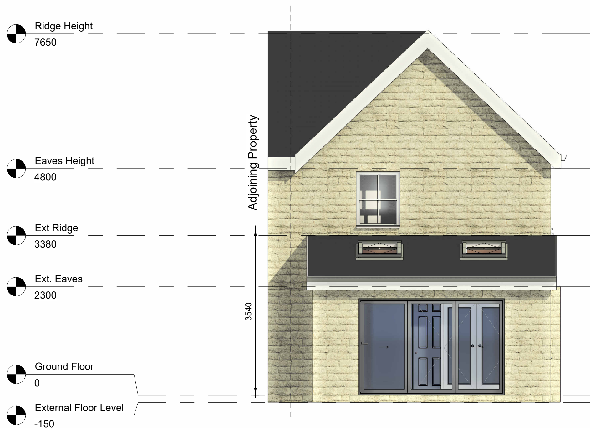
3 Proposed LHS Gable Elevation 1 : 50
