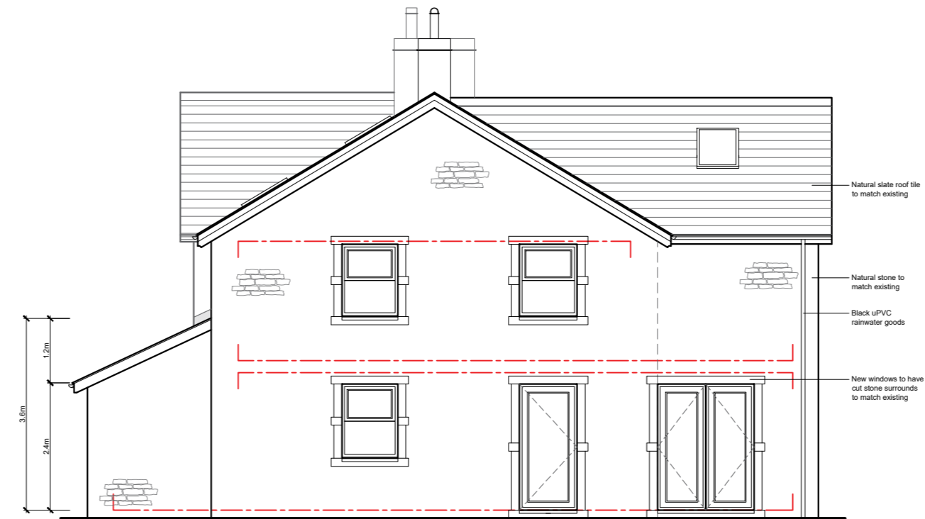
Proposed South East Facing Elevation Scale 1:100
