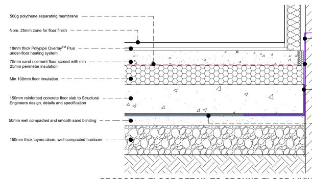
PROPOSED FLOOR DETAIL TO GROUND FLOOR LIVING ROOM (DETAIL TO BE READ IN CONJUNCTION WITH CORDEK DETAILS) SCALE: 1:10
