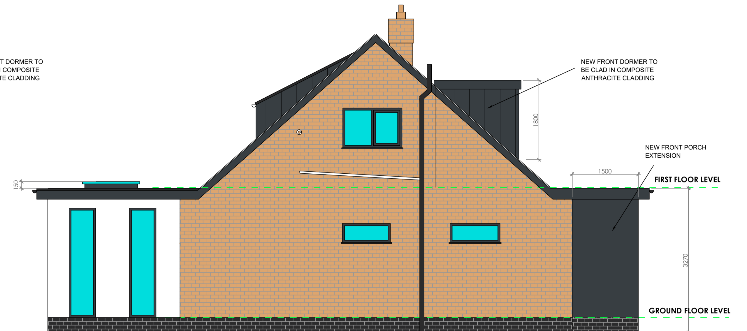
PROPOSED SIDE ELEVATION SCALE - 1:50 @ A1
