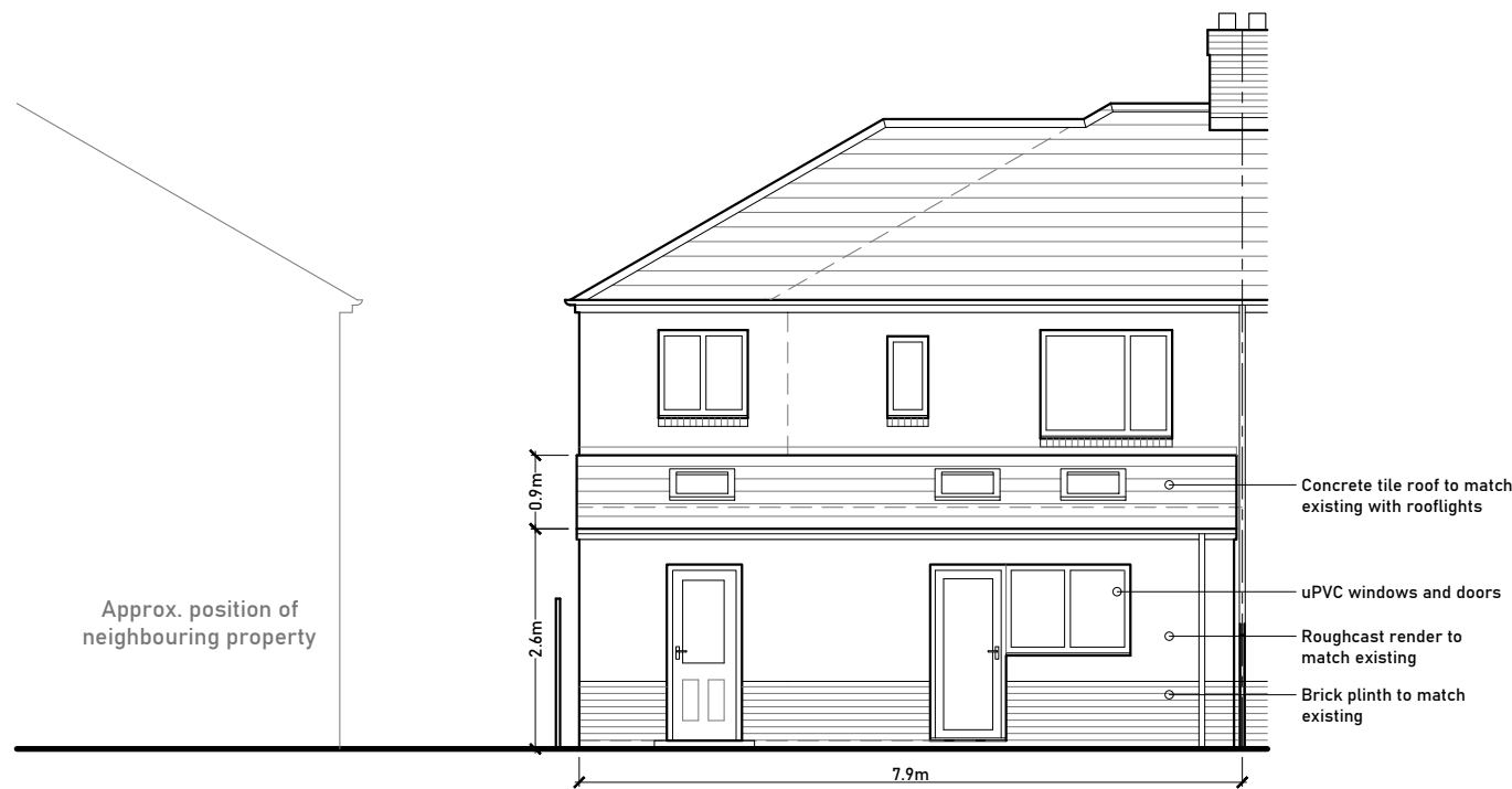
NORTH WEST ELEVATION
