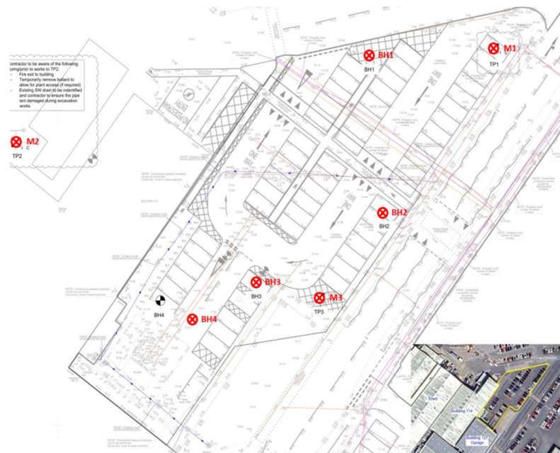
Fig 5.4 Borehole and trial pit location plan
