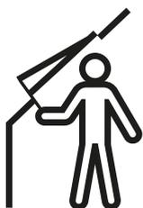
The Heritage conservation roof window GCL is a top-hung window that is operated with a hand-winder fixed to the bottom frame. The window can be opened to a maximum of approx. 150 mm. The black profiles, central glazing bar and flashing beautifully match historical buildings.
