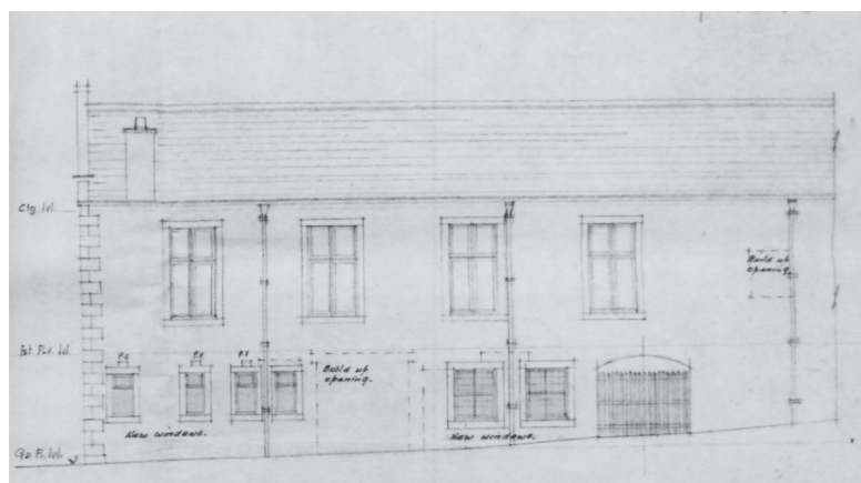
Elevations from 1962 showing the proposed, the existing is shown hatched
