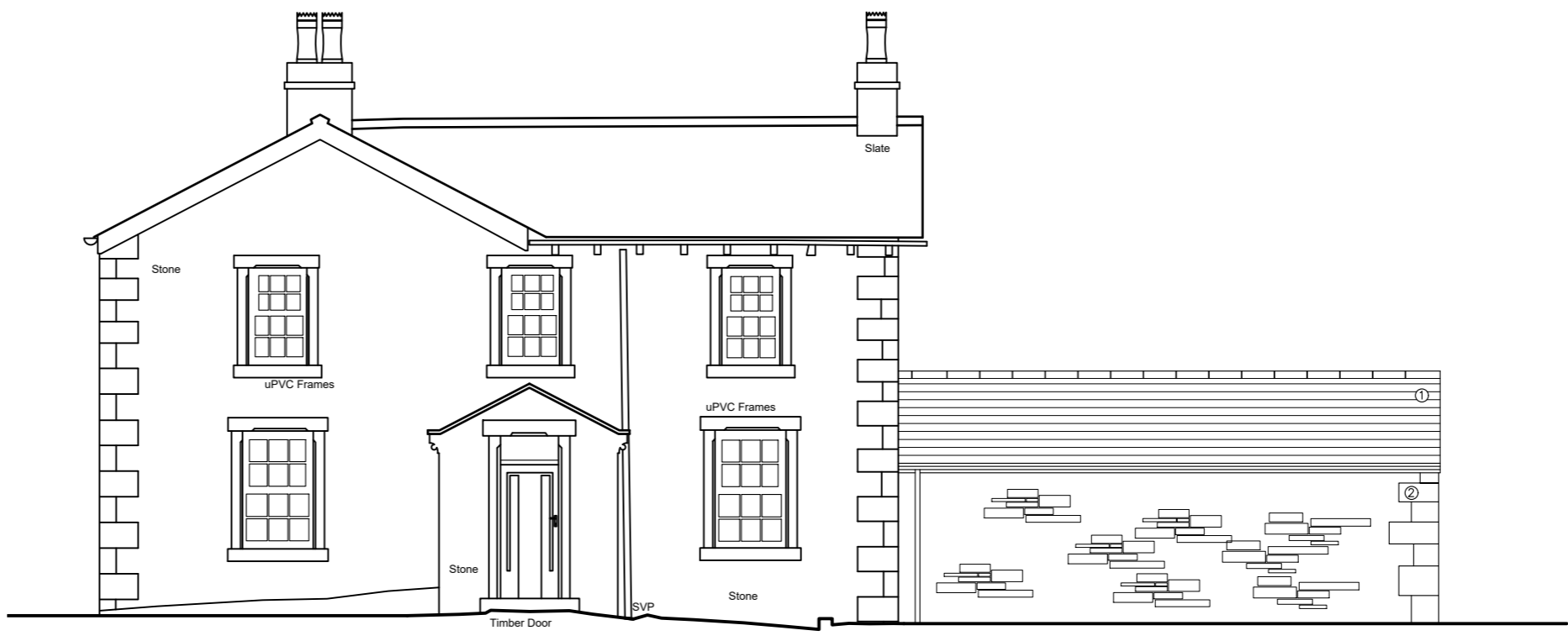
PROPOSED FARMHOUSE (GARAGE 1) NORTH EAST ELEVATION (9)
