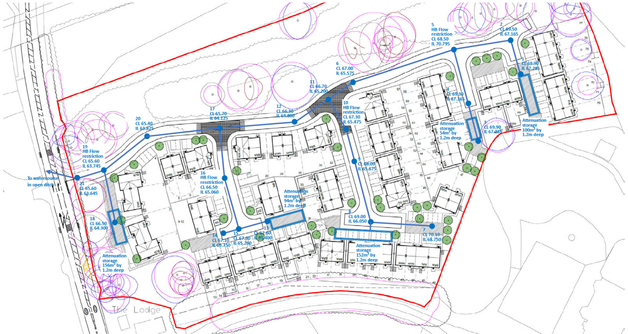
SURFACE WATER DRAINAGE LAYOUT
