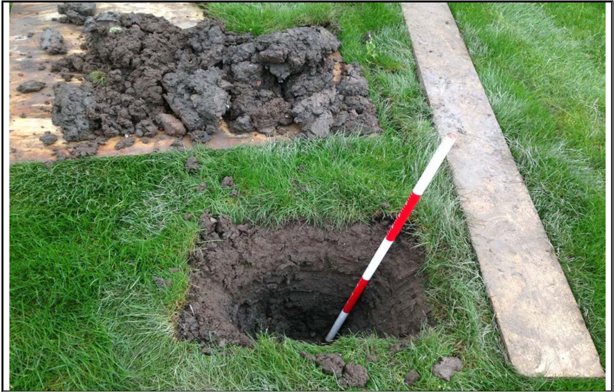
Plate 3 – Plot No 15 Cover System Depth & Arisings
