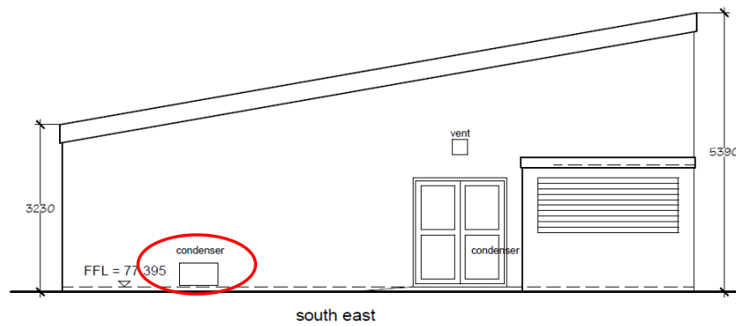
Figure 4 Location of new condenser unit
