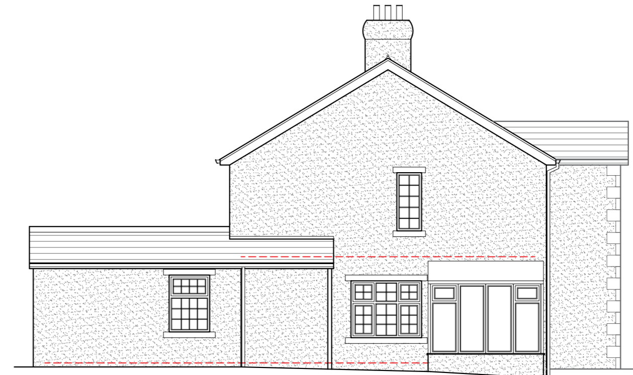
Existing South West Facing Elevation Scale 1:100
