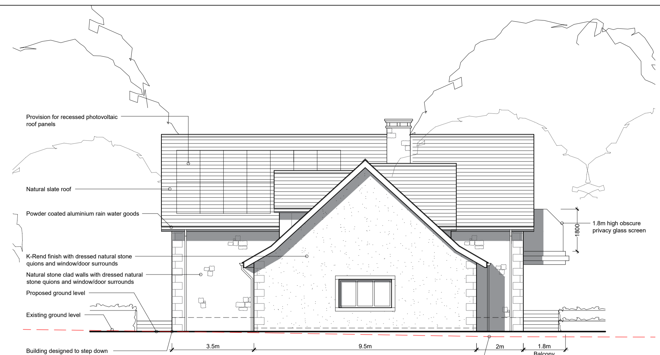
South East Elevation Datum +112.00
