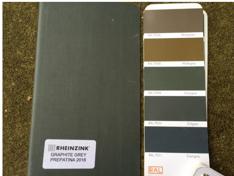
Pl. 4 Photo showing Rheinzink Graphite Grey Zinc sample for dormer wall cladding and walls above the stone string and garage flat roof. This is shown next to the RAL 7010 swatch for window and door frames and rainwater goods.
