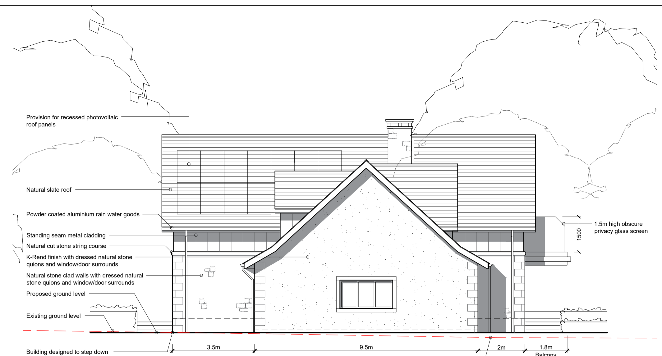
South East Elevation Datum +112.00
