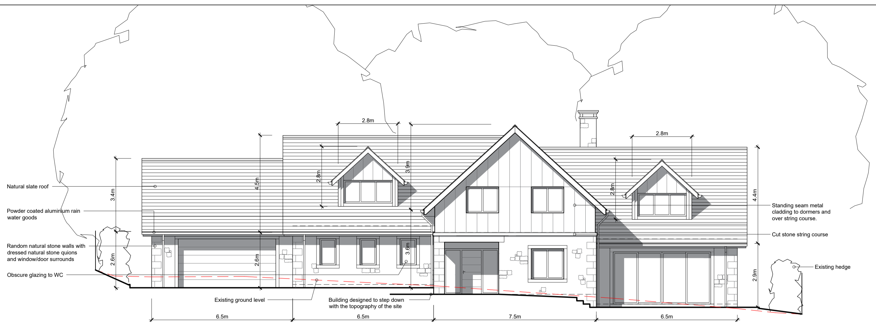
South West Elevation Datum +112.00
