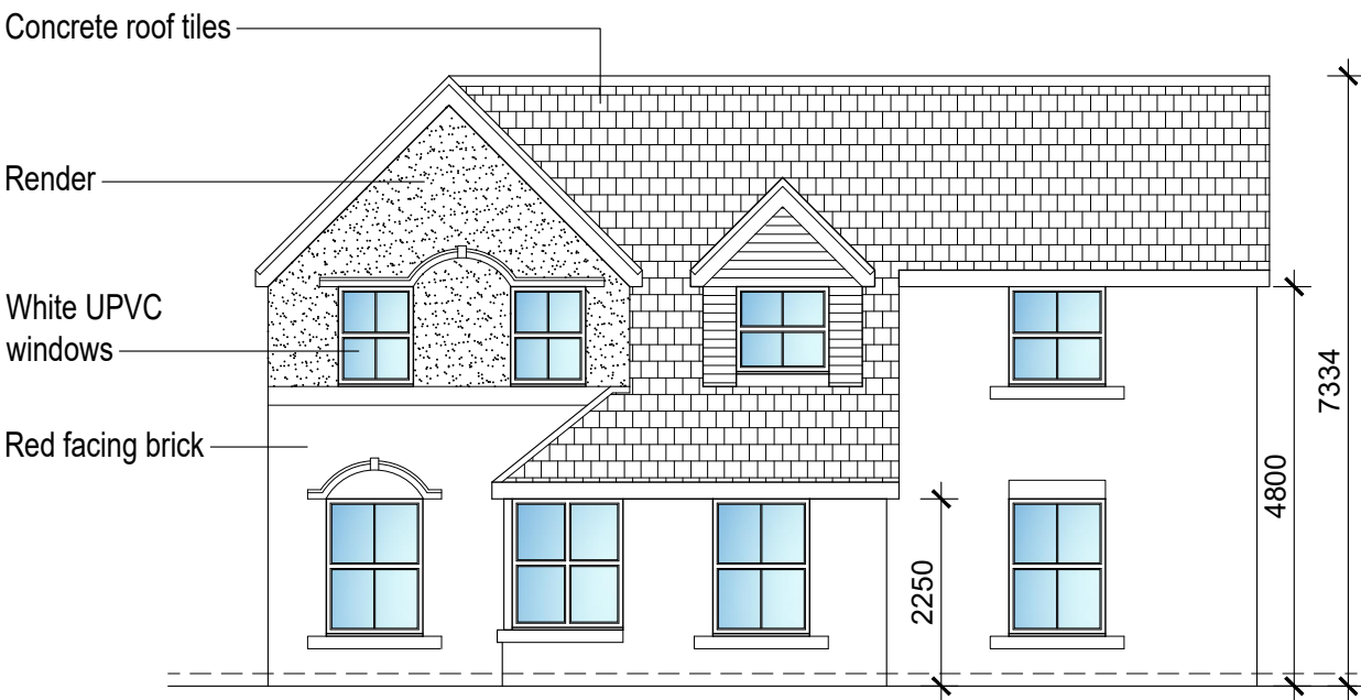
Existing South West Elevation
