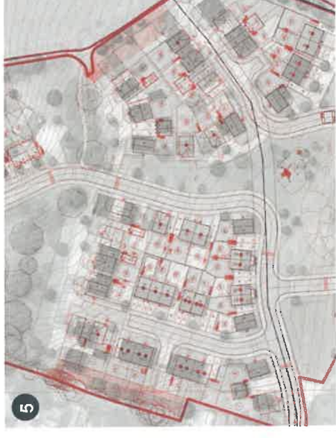
Response to para. 20 showing amendment to rear gardens to plots 4-8 to replace retaining wall with earthworks battering in this area to assist with relationship to existing dwellings and allow for retention of existing trees.
