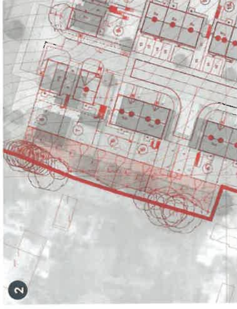
Response to para. 20 showing amendment to rear gardens to plots 4-8 to replace retaining wall with earthworks battering in this area to assist with relationship to existing dwellings and allow for retention of existing trees.
