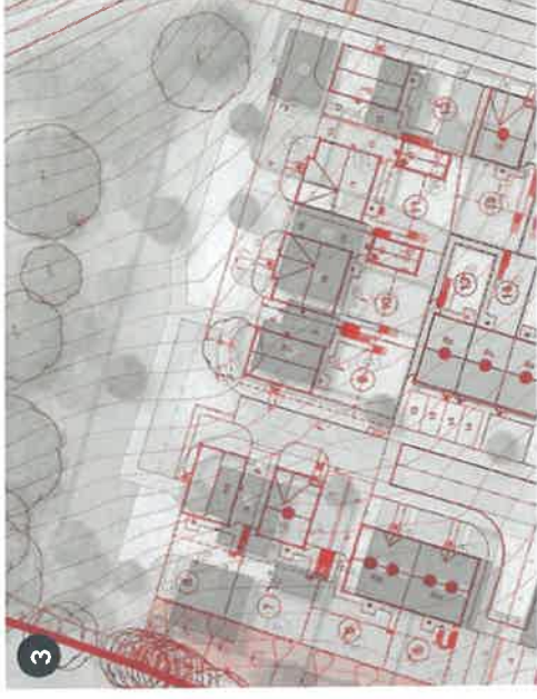
Response to para. 21 showing revised layout and arrangements to plots 8-12 with revised retaining walls to provide a continuous building line and prevent the creation of an overbearing boundary feature.
