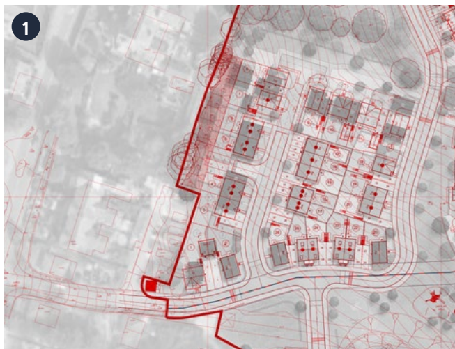
Response to para. 19 showing reconfiguration of western boundary plot arrangement to increase landscape buffer and improve relationship with existing properties.
