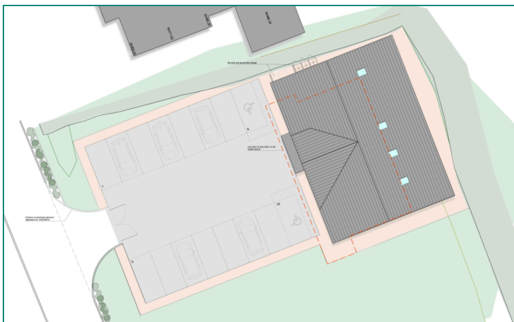
Figure 6 - Proposed Site Layout Plan with hatched red line showing position of existing building
