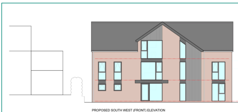
Figure 7 - Proposed front elevation showing height relative to neighbouring building
