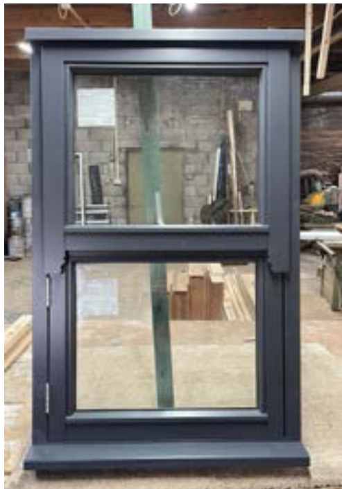
Mock Sash Timber Windows - Windows being painted White.
