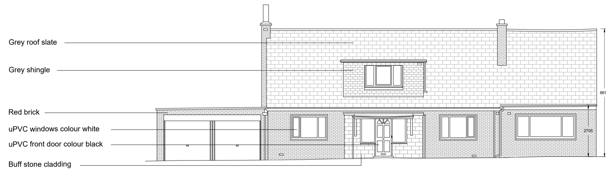
Existing South-West Elevation Scale 1:100
