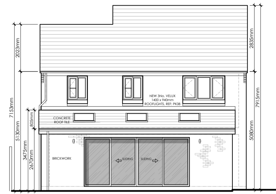
PROPOSED REAR (SOUTH EAST) ELEVATION Scale 1:100
