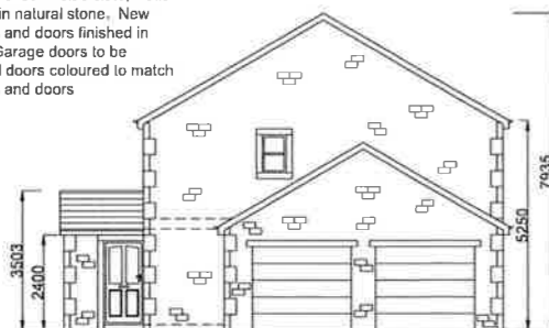
PROPOSED GABLE ELEVATION SCALE 1:100
