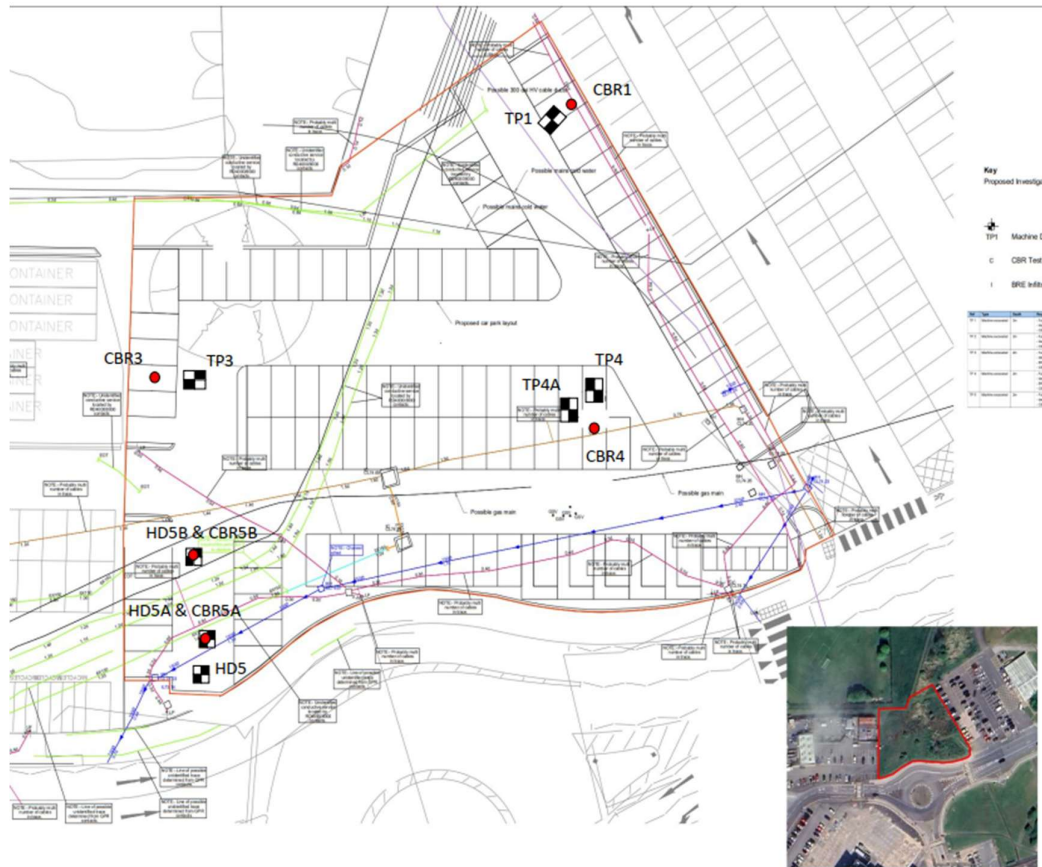
Fig 5.4 Borehole and trial pit location plan
