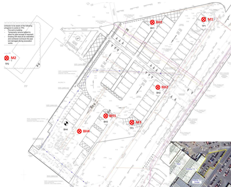
Fig 5.4 Borehole and trial pit location plan
