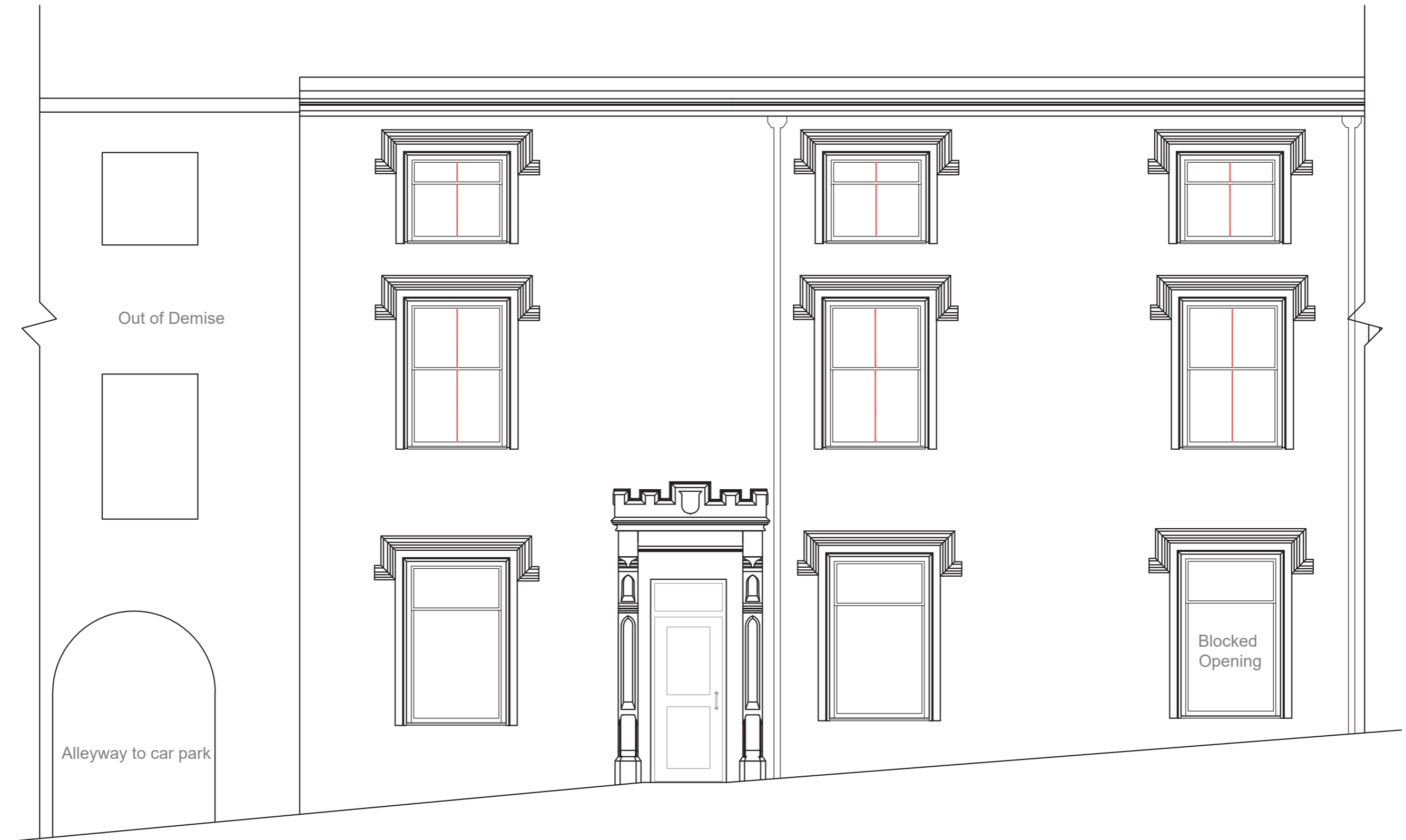
EXISTING SHOPFRONT ELEVATION SCALE 1:50
