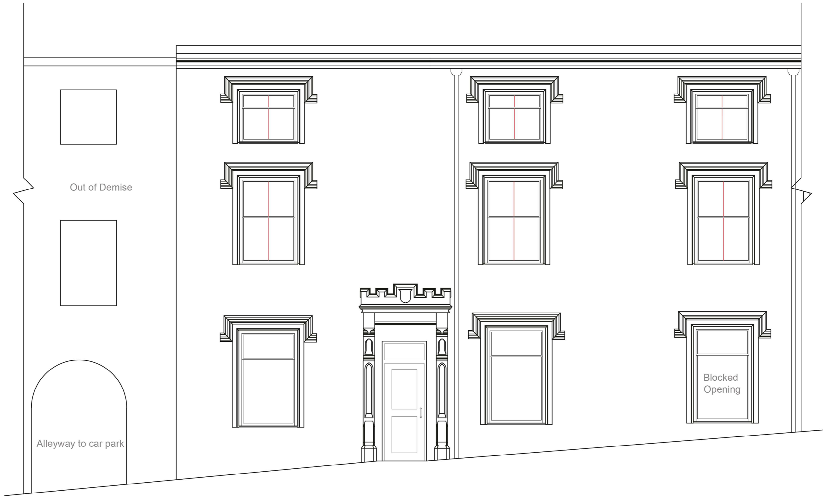
EXISTING SHOPFRONT ELEVATION SCALE 1:50
