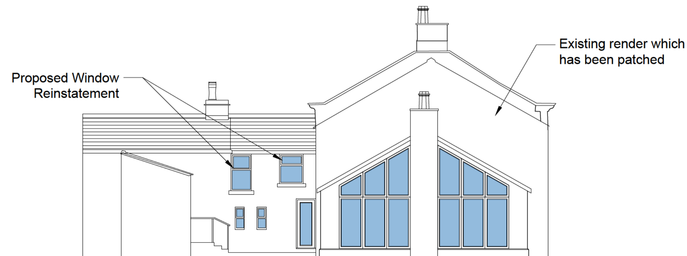
Proposed South West Elevation Scale 1:100 @ A1
