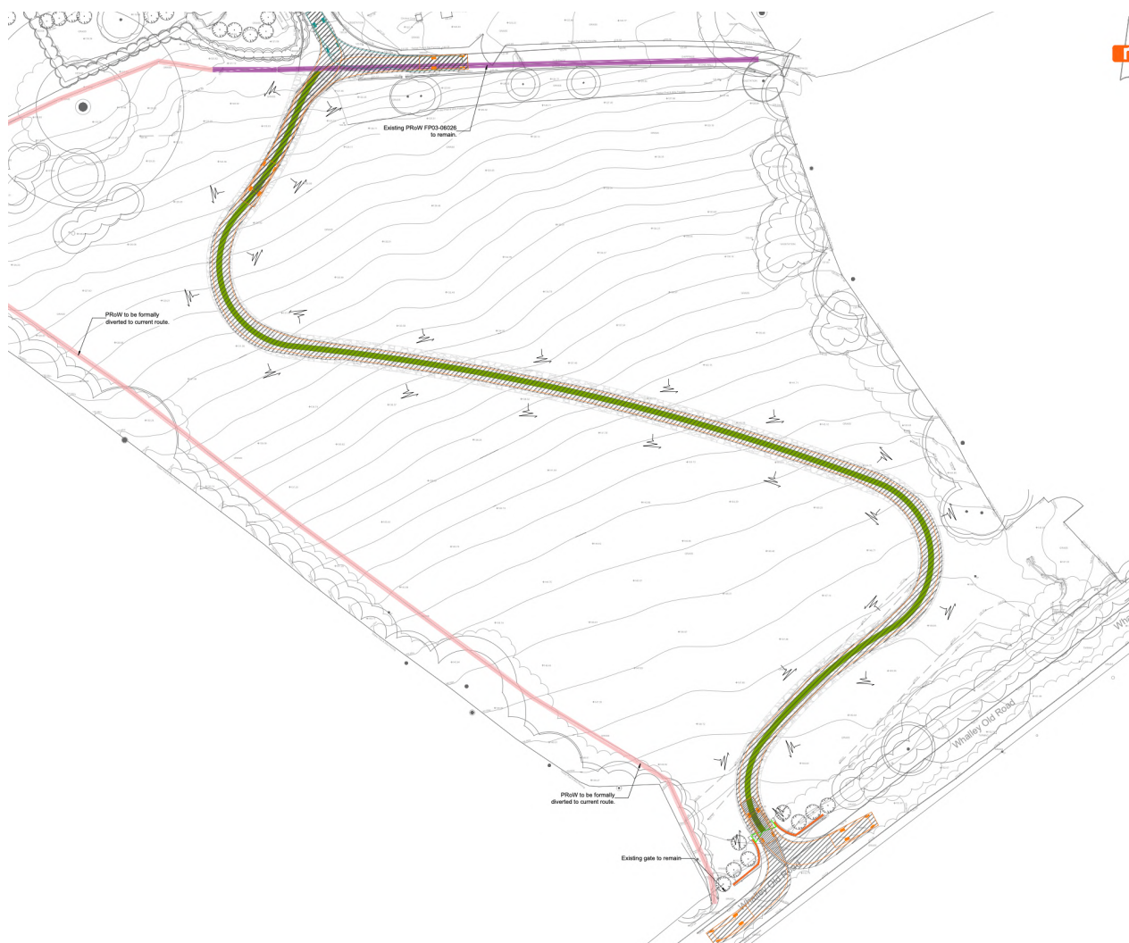
Figure 3.3 : Swept Path Analysis – 7.5t Box Van (source: Mode Infrastructure)
