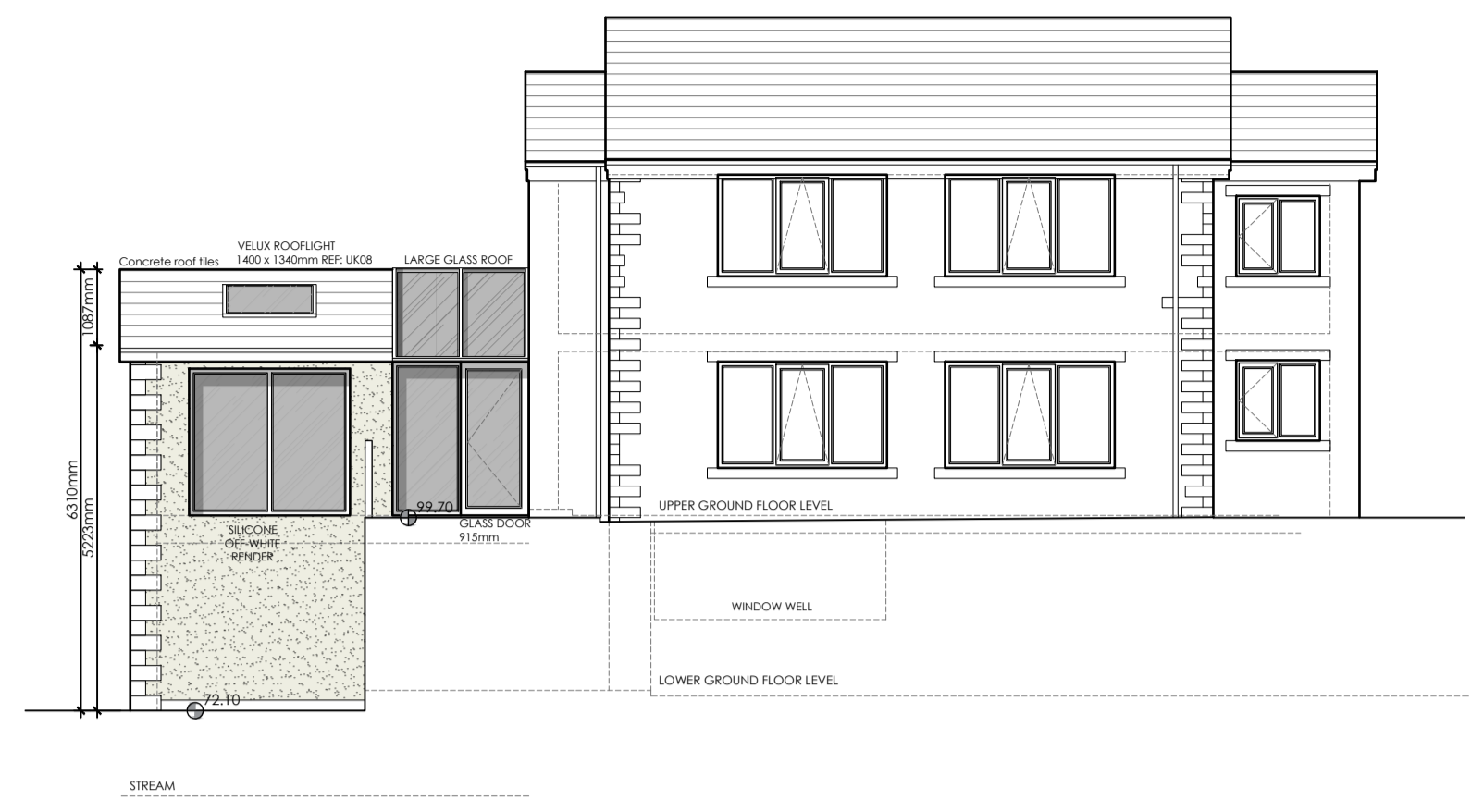
PROPOSED SIDE (SOUTH) ELEVATION Scale 1:100
