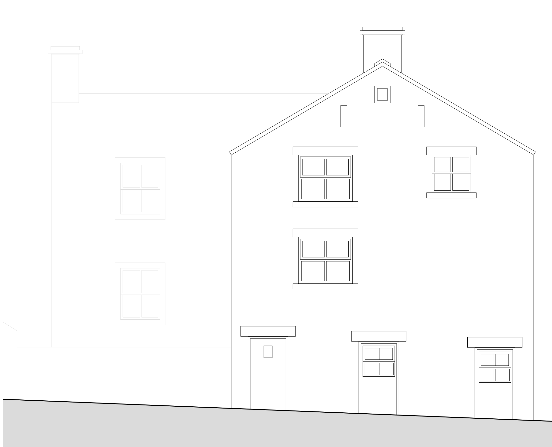
Front Elevation as EXISTING 1:50
